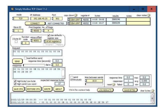
The PMC-1 uses the ModBus TCP protocol for data communication. The ModBus TCP protocol is inherently insecure, meaning it does not support encryption or user authentication (passwords).
