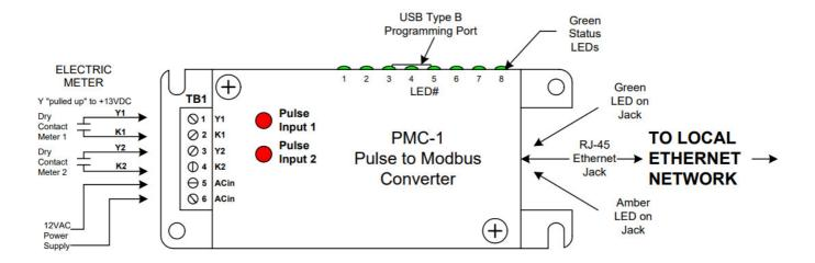
**MOUNTING POSITION** – The PMC-1 can be mounted in any position. Two mounting holes and 2 slots are provided.
