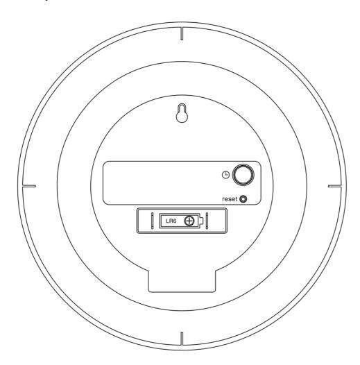
Insert 1xAA (1.5V) battery observing the correct polarity, as shown on the diagram.
