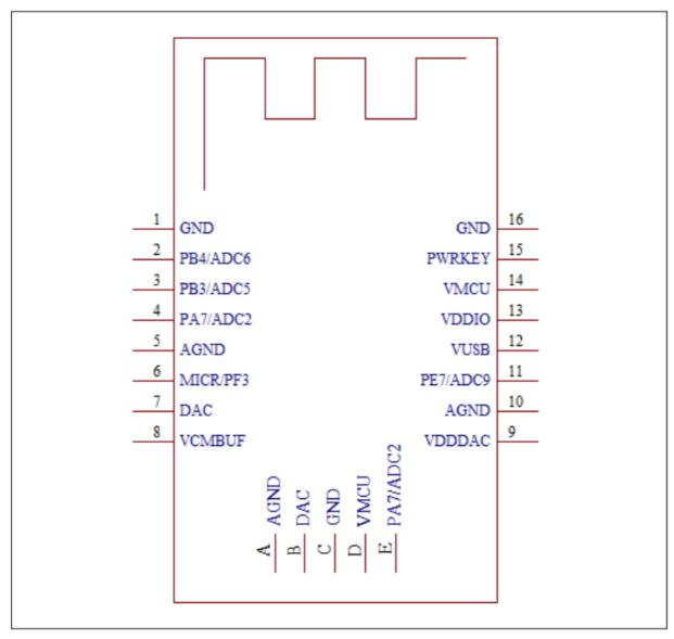
Figure Pin assignment for M8020A
