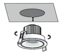
4. Fold up the retention clamps and press the luminarire through the hole. Make sure the clamps grip to the ceiling and that the luminaire or driver is not covered with thermally insulating material.
