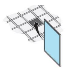
3. Make sure to angle the luminaire to get it through the ceiling opening.
