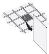
2. Lift the luminaire through the ceiling opening.
