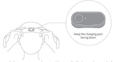
2. Tighten the headband properly into an appropriate position, until all electrodes are in full contact with the skin.
