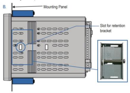
• C. Insert curved tab of retention brackets(C) into notches in the top, bottom and sides of the MCT(B) and tighten screws evenly in order to secure the MCT in place.
