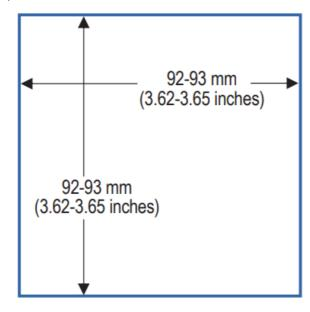
• B. Insert MCT controller through front panel cutout.
