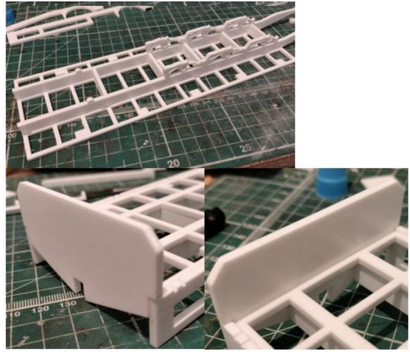
• **Step 7**: Fit the side assemblies. Align the front end with the notch in the headboard, the rear should sit flush on the tops of the part 7's you glued on in step 1. This should leave the entire side approx. 1mm higher than the floor. Repeat for both sides.
