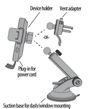
Join the device holder with either the dash/window mount or vent adapter ,,,
