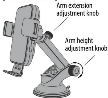
For taller or shorter phones, move the foot on the device holder up or down to properly align your phone with the wireless charger. This adjustment will be different for every phone model. Your phone will start charging when it is in proper alignment. Aligning the wireless charging components correctly will allow your phone to receive the fastest charge possible.
