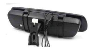
**Step 2**Route the wiring from the back of the mirror into the vehicle headlining and run it towards the passenger side of the vehicle.
