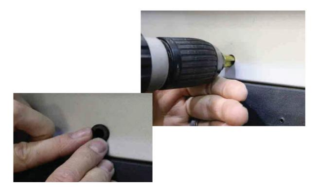
**Step 9**Next, run the cable through into the area behind the license plate and then mount the bracket tightly.
