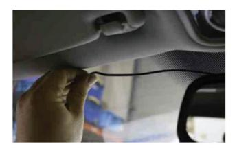
**Step 3**Continue running while the harness is down the A-pillar of the vehicle while taking care not to obstruct or impede any vehicle airbags. The wiring harness should always be routed behind the airbag rather than in front of it.
