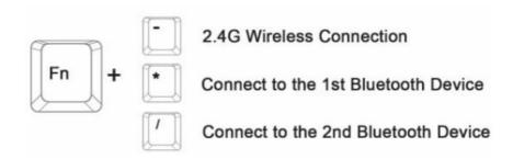
After following the above steps to connect, you can short press the right key combination to switch to the connected device for use.
