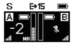
• From the Home screen, press the power button to access the options of the A or B channel gain and output volume in turn→ press the M button to adjust the value → press the power button again to save the setting.
