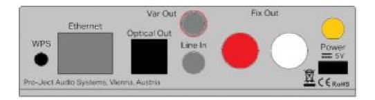
Make all connections whilst the preamplifier is disconnected from the power supply.
