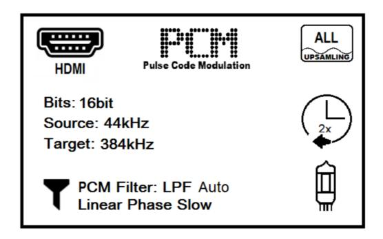
HDMI input (CD Box RS2T) PCM data on input Upsampling active Bit depth of incoming signal: 16bit Sampling frequency of incoming signal 44kHz sampling frequency of converted signal 384kHz Filters set to LPF Auto and Linear Phase Slov Reclocking set to 2x Tube stage active
