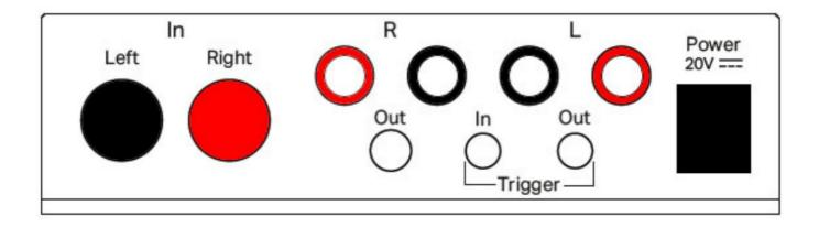
Make all connections whilst the amplifier is disconnected from the mains. Take care to connect the left and right channels correctly. The right channel is usually marked red, the left channel black or white.
