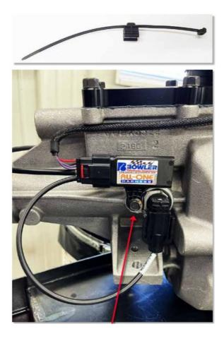
The epoxy sealed control module should be attached to the transmission using the bolt that fastens the speed sensor clamp. Do not overtighten this bolt.
