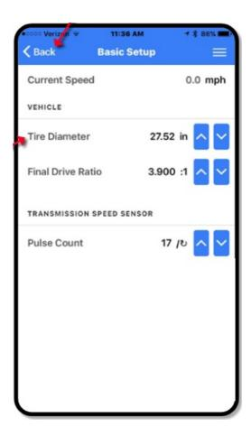
The Basic Setup screen allows you to input the specifics needed for the All-In-One unit to correctly interpret the information it is sending.
