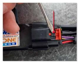
The All-In-One harness has a built-in fuse located near the reverse switch connector. This is a 3 amp fuse to protect the circuit board inside the controller. Removal of the fuse link or swapping to a larger fuse size will void any warranty. We recommend using a zip tie and attaching it to the empty case hole directly above the reverse light connector.
