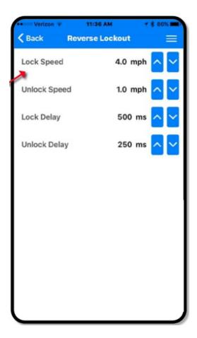
There is really no reason to change any settings on the Reverse Lockout Solenoid. The default settings are recommended, which will allow the shifter to easily go into reverse from 0-4 mph and will have the spring detent to make going into reverse difficult above 5 mph.
