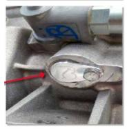
The main controller and harness can be separated for service or installation reasons. To disconnect the harness simply slide the red tab away from the connector, then press down on the small black tab while gently pulling the connector away from the controller.
