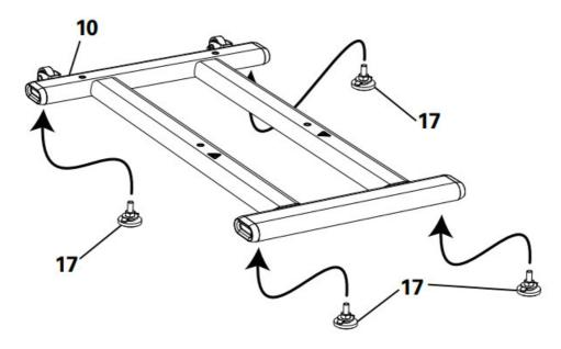
2. Attach Rail Assembly to Frame and then Release the Frame from the Shipping Plate
