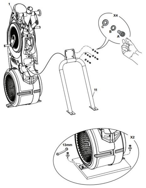
3. Carefully Lift the Frame Assembly from the Shipping Plate and Attach to the Stabilizer Assembly
