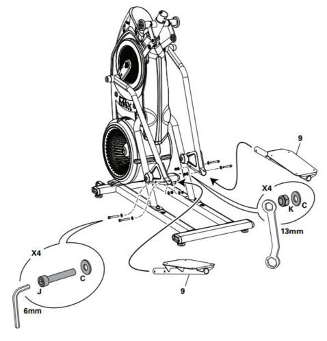
7. Attach the Foot Platforms and then the Foot Pads to the Pedals
