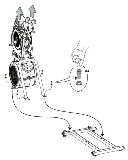
4. Attach Rear Shroud and Caps to the Frame Assembly
