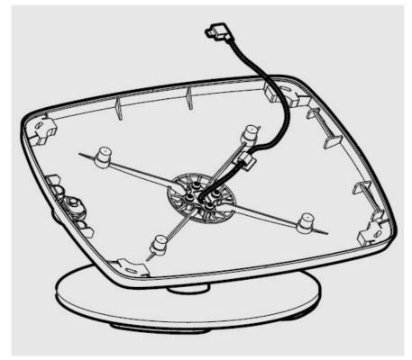
• Feed the tablet cable through the Bouncepad Case & mounting arm.
