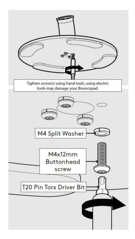
• Locate & secure the Flex Mounting Arm to the Freestanding Base.
