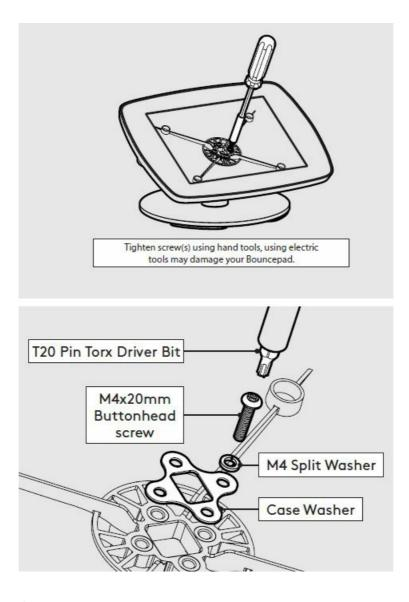
• Attach the Bouncepad Case to its Mounting Arm. Take care to ensure correct & full thread engagement.
