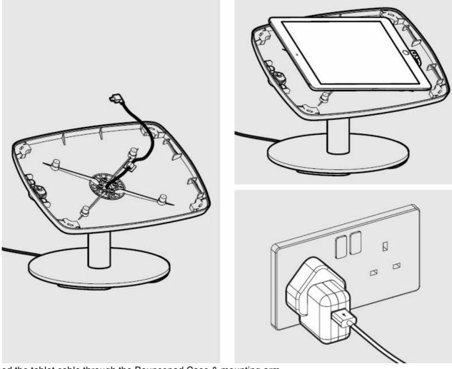
• Feed the tablet cable through the Bouncepad Case & mounting arm.
