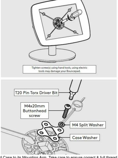
• Attach the Bouncepad Case to its Mounting Arm. Take care to ensure correct & full thread engagement.
