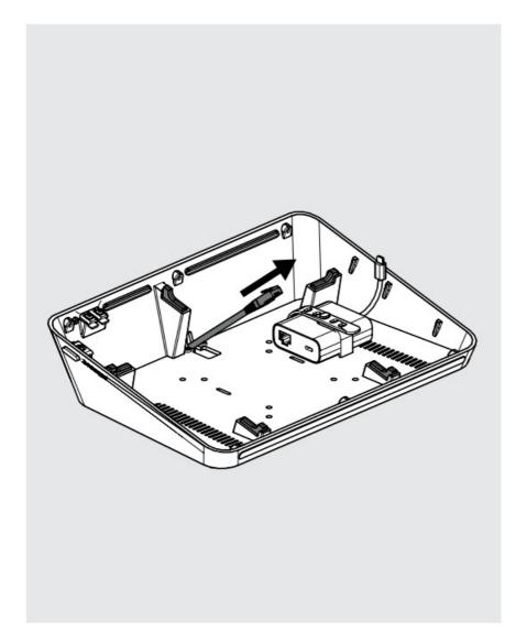
8. Connect the ethernet cable to the POE and secure the cable with the cable lock.
