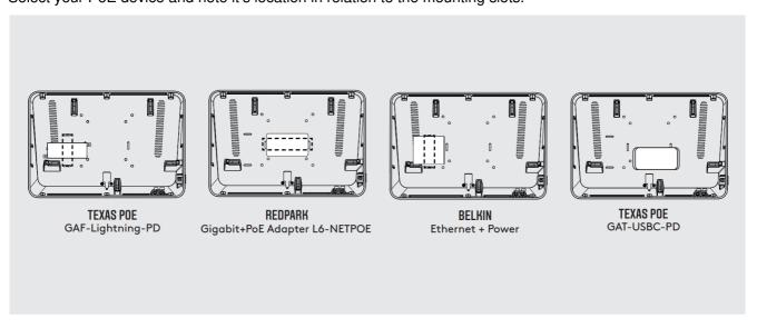
5. Insert the tie through the cable slots and then clasp over the POE device.
