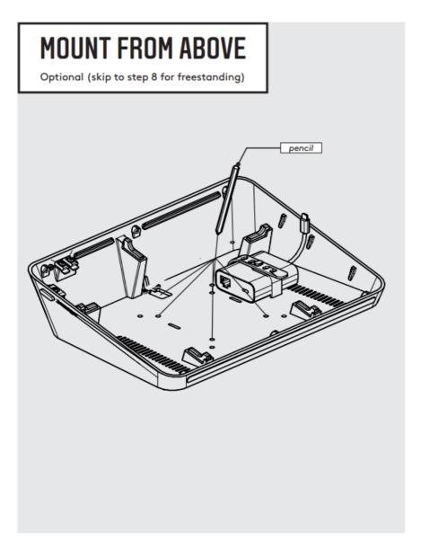
**A2:** Use a drill bit suitable for your surface and make 4x pilot holes.
