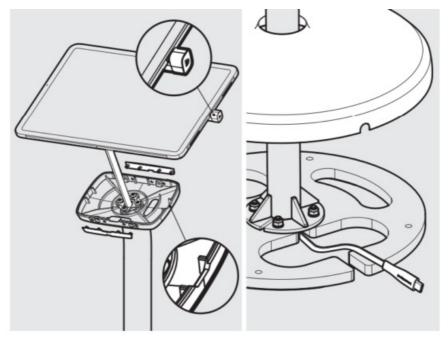
Secure the Tablet to the Shell & attach the Fixing Covers as shown.
