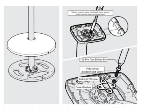
Remove the Mounting Plate adhesive backing. Attach level & centrally to the Tablet back as shown.
