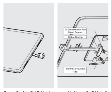
Remove the Fixing Covers. Feed the Flat Cable into the assembly & locate the Tablet in the chosen orientation.
