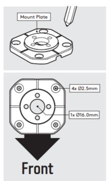
• Using the Mount Plate, mark the drill hole locations as shown.
