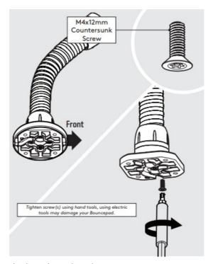
• Join the Flex Arm & Mount Plate in the orientation shown.
