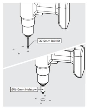
• Drill each hole – using the specified drill sizes.
