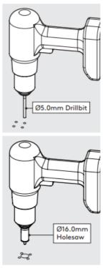
• Drill each hole – using the specified drill.
