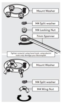
• Secure the arm to the surface. Locking Nuts offer higher security.
