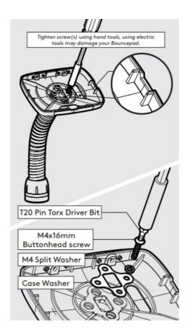
1. Locate & attach the Shell to the Flex in the correct orientation.
