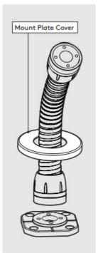
• Locate the Cover onto the Flex.
