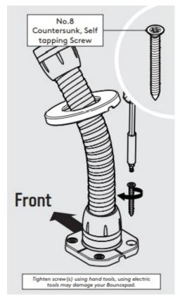
• Secure the Flex to the surface with the 4x countersunk fixings.
