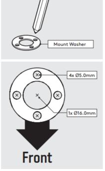
• Using the Mount washer, mark the drill hole locations.
