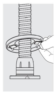
• Adhere the Mount Cover onto the Mount Plate with the adhesive tabs.
