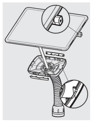
5. Remove the Fixing Covers. Feed the Flat Cable into the assembly & locate the Tablet in the chosen orientation.
