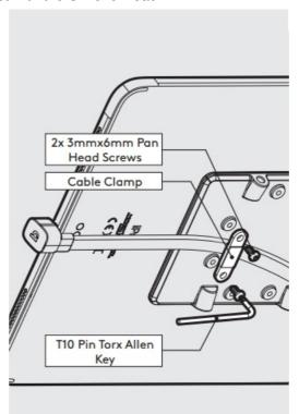
4. Secure the Flat Cable to the Mounting Plate with the Cable Clamp as shown.
