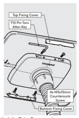
Secure the Tablet to the Shell & attach the Fixing Covers as shown.
