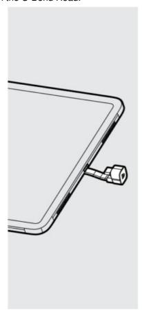
5. Secure the Flat Cable to the Mounting Plate with the Cable Clamp as shown.
