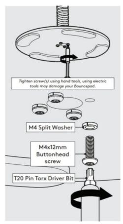
2. Locate & attach the Shell to the Flex in the correct orientation.
