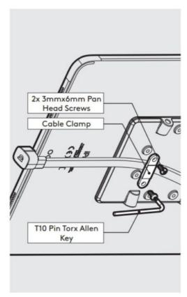
6. Remove the Fixing Covers. Feed the Flat Cable into the assembly & locate the Tablet in the chosen orientation.
