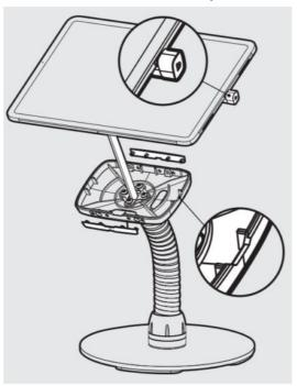
7. Secure the Tablet to the Shell & attach the Fixing Covers as shown.
