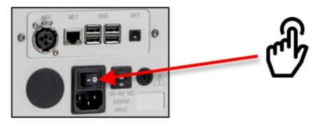
2. Insert the USB receiver into one of the USB connectors on the rear panel. It does not matter which USB connector you choose.
