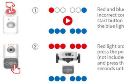
Red and blue indicator light flash alternately: Incorrect command use. Please press the start button once to correct the error until the blue light is on.
