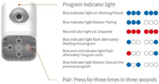
to pair with Botzees main control block before first use. If paired, the device will be automatically connected at next time.
