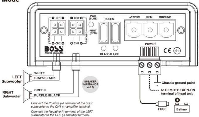
Connect the Positive (+) terminal of the RIGHT subwoofer to the CH3 (+) amplifier terminal.
