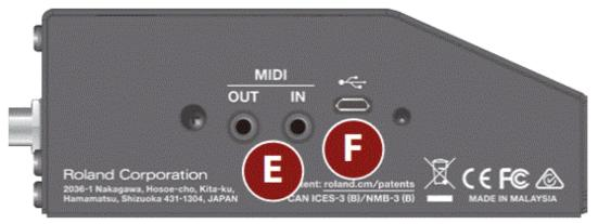
Connect an external MIDI device here. You can synchronize an external MIDI device with this unit.
