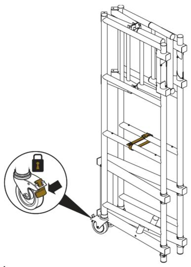
• Unfold sides of the frame
