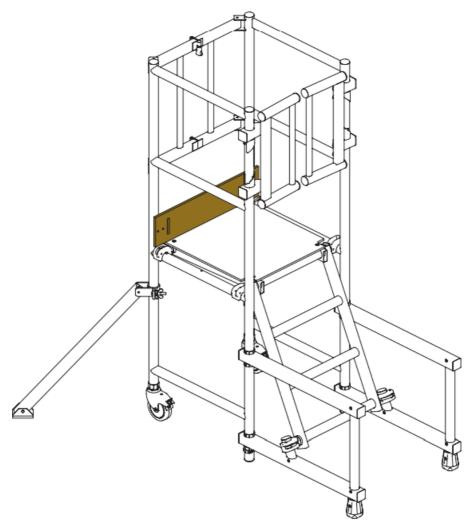
2. Slide the first side toe board into the slot of the front toe board. Push the clip on to the rear vertical tube as shown. Ensure the side toe board is in contact with the surface of the platform. Note: The toe board fits on the inside of the BoSS Pod2 frame.
