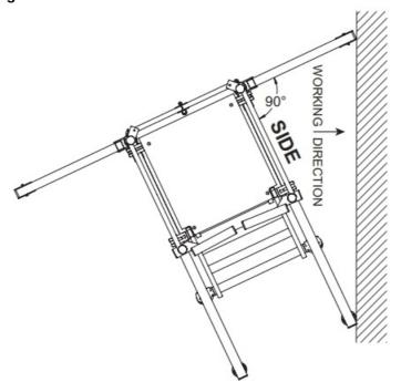
The stabilisers must be correctly deployed, as shown above, before use.
