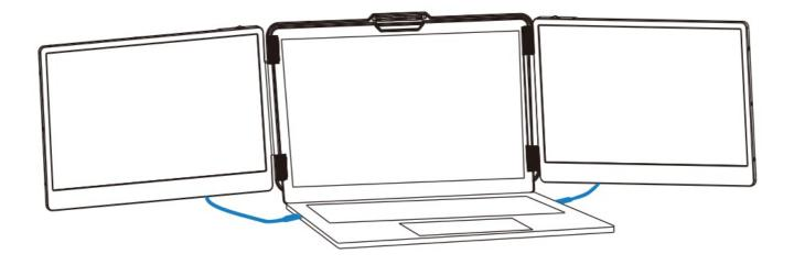
Connect to S2 through the Type-C interface of the notebook Option 1: If your laptop has two Type-C ports (full function ports), and the Type-C output port of the laptop can provide more than 5V/2A power supply, directly connect the S2 and the laptop with two Type-C cables.
