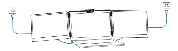
Option 2: If your laptop has 2 Type-C ports (full function ports), and your laptop Type-C outlet cannot provide more than 5V/2A power supply or the display has no signal/the signal is unstable after connection, then you need to connect an external 5V/2A adapter to power S2. Then connect the S2 to the laptop with two Type-C cables.
