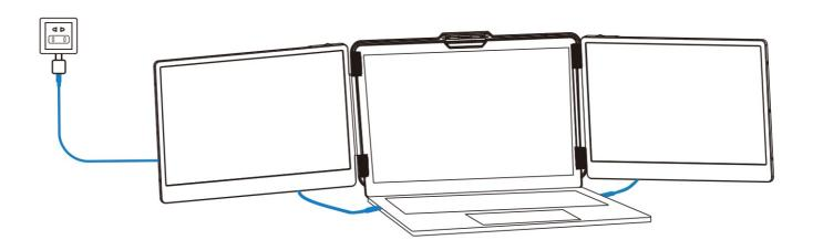
To connect the S2 screen to your laptop via the HDMI interface, follow these steps: Option 3: If your laptop has both a Type-C and an HDMI port, you can use a Type-C cable to connect the S2 screen to the Type-C port of your laptop, and then use an HDMI TO TYPE-C cable to connect the S2 screen to the HDMI port of your laptop. After that, you can connect a 5V/2A adapter to power the S2 screen.
