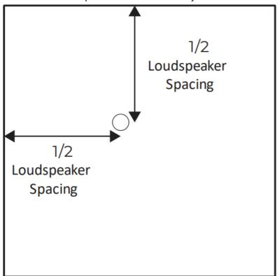
The remaining loudspeakers are arranged on a square grid pastern using the LSD. If a loudspeaker would be placed on or beyond the perimeter of the room, delete that row/column of loudspeakers.
