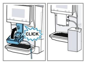
15. Connect a carton of milk to the milk inlet tube and the suction pipe. Note: Fill the water tank each day with fresh, cold, non-carbonated water. Tip: To keep the coffee beans at their best, store them in a sealed container in a cool place. You can keep the coffee beans in the bean container for several days without them losing their aroma
