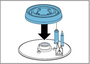
4. The catching pin on the outer ring cap must fit into the corresponding slot on the burner head.
