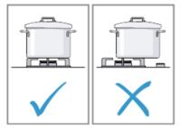
Place cookware onto the pan supports. Never place cookware directly on the burner. Before using the appliance, ensure that the pan supports and gas burner caps are positioned correctly.
