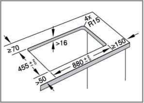
The angle between the cut surface and the worktop must be 90°.
