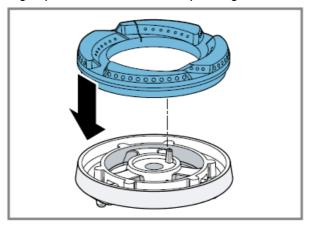
5. The catching pin on the inner ring cap must fit into the corresponding slot on the burner head.
