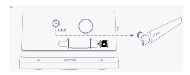
**A** Insert LTE antenna 1 into LTE antenna 1 port and rotate the antenna nut in a clockwise direction until it is firm. Ensure not to overtighten.
