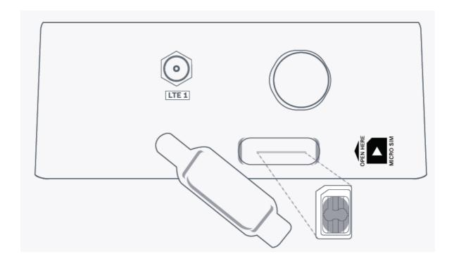
Insert Micro SIM into Phantom Edge as per the marking sticker
