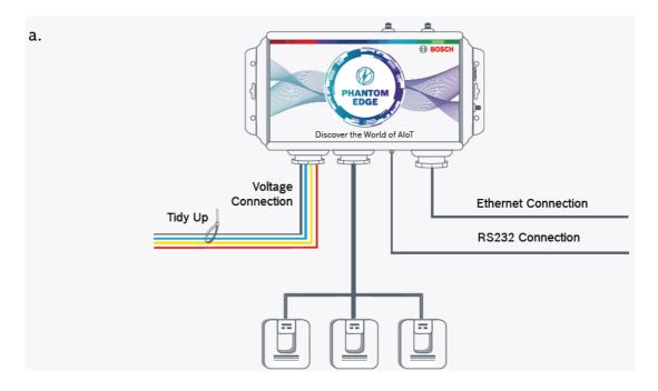
A Use the cable ties to secure and bundle the cables
