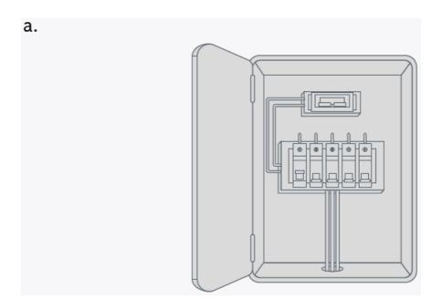
**B** Remove approx. 50mm of insulation from wires. Connect the four-individual wire strands in the voltage connector cable to the appropriate points of the four-pole MCB. Follow color coding of the wire strands to ensure correct connection (Refer exhibit 1).
