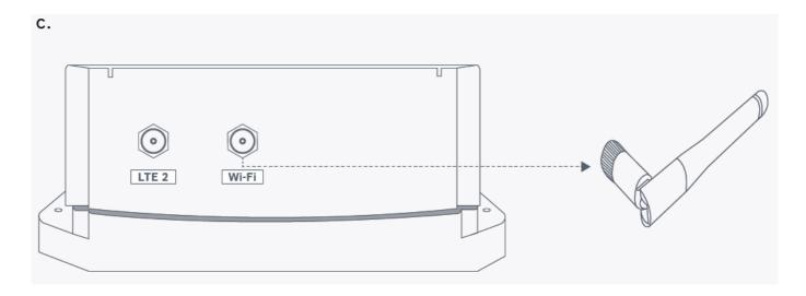
**C** Insert Wi-Fi antenna into Wi-Fi antenna port and rotate antenna nut in a clockwise direction until it is firm. Ensure not to overtighten.
