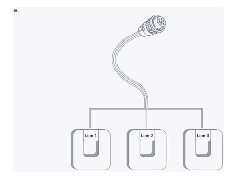
**B** Clamp CT around the individual power cable for each phase. Ensure that the front surface of the CT and line label, is oriented in the direction of power source. Ensure color code of the power cable and line label matches. (Refer Exhibit 1)
