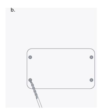
**A** Use the Drill Paper Guide and mark the four locations to drill on the target wall **B** Drill holes of sufficient depth to accommodate wall plugs provided in the installation kit
