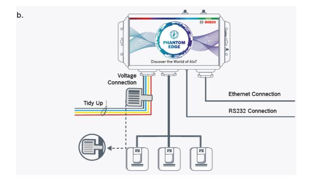
**B** Fill in the contact details of local technician and tag it on the voltage cable. Ensure all details are correctly filled for emergency response.
