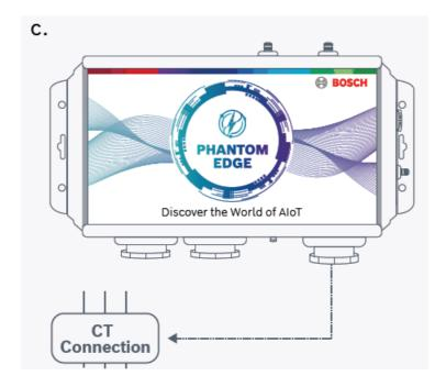
**C** Mount Phantom Edge in a horizontal direction by using adhesive surface of the stickers. Ensure mounting surface is cleaned using Iso-Propyl alcohol before sticking the device.
