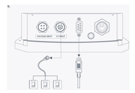
Connect machine PLC RS232 female connector to the male connector of Phantom Edge and tighten the screws
