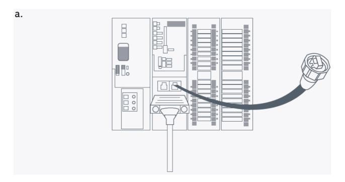
Identify the recommended Amphenol RJ45 Cable RCP-5SAMMM-SLM7Bxx male connector connected to machine PLC
