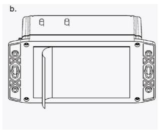
A Clean the backside of the device using Iso-Propyl alcohol, peel off the liner from one side of double sided tape and stick it to the backside of Phantom Edge as shown above. Ensure there are no air bubbles while sticking.
