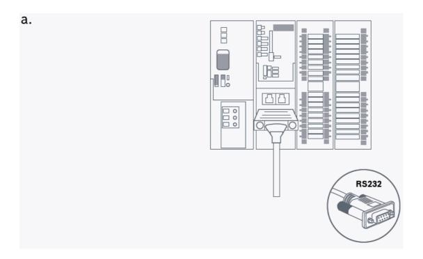
Identify RS232 female connector connected to machine PLC
