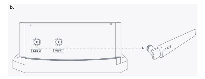
**B** Insert LTE antenna 2 into LTE antenna 2 port and rotate the antenna nut in a clockwise direction until it is firm. Ensure not to overtighten.
