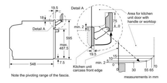
If the applience will be installed underneth a hold the following worktp thickness including substructer if necessary must be taken into account.
