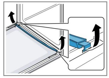
8. Lift out the intermediate pane and set it down carefully on a flat surface.
