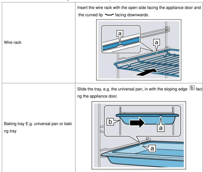
3. Push the accessory all the way in, making sure that it does not touch the appliance door.
