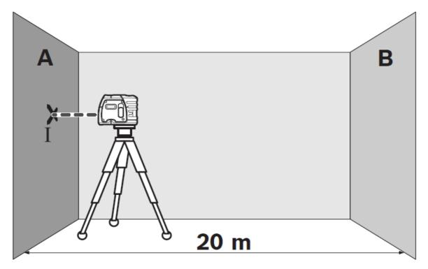
• Direct the horizontal laser beam, which runs parallel to the longitudinal axis of the measuring tool, at the close wall A
