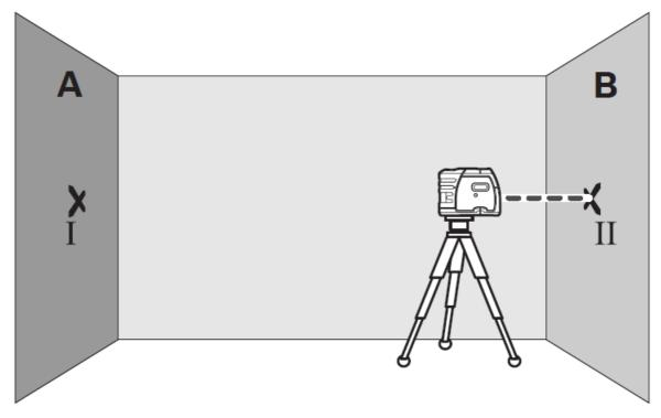
• Align the height of the measuring tool (using the tripod or by underlaying, if required) in such a manner that the centre point of the laser beam is projected exactly against the previously marked point II on wall B.
