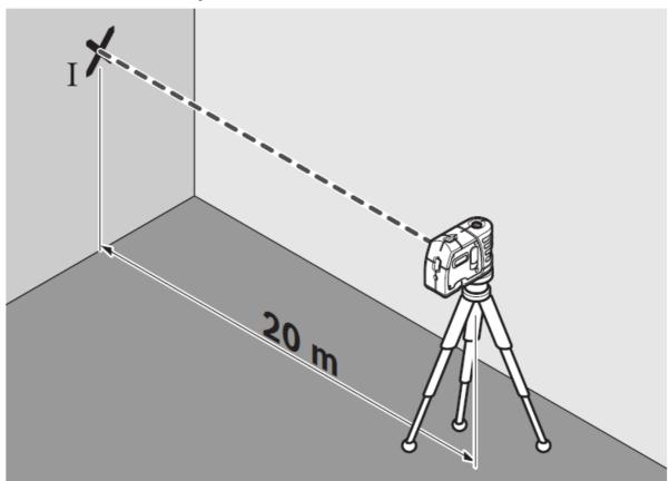
• Direct one of the two lateral laser beams, that run alongside the lateral axis of the measuring tool, at the wall. Allow the measuring tool to level in. Mark the centre of the laser beam on the wall (point I).
