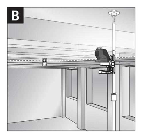
Use the laser receiver 26 to improve detection of the laser lines in adverse lighting conditions (bright environment, direct sunlight) and over greater distances. Switch on receiver mode when working with the laser receiver (see "Receiver mode", page 20).
