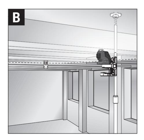
With the universal holder 24, you can fasten the measuring tool, e.g., to vertical surfaces, pipes or magnetisable materials. The universal holder is also suitable for use as a ground tripod and makes the height adjustment of the measuring tool easier.
