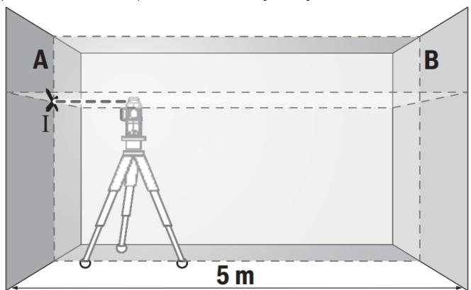
• Direct the laser against the close wall A and allow the measuring tool to level in. Mark the centre of the point where the laser lines cross each other at wall A (point I).
