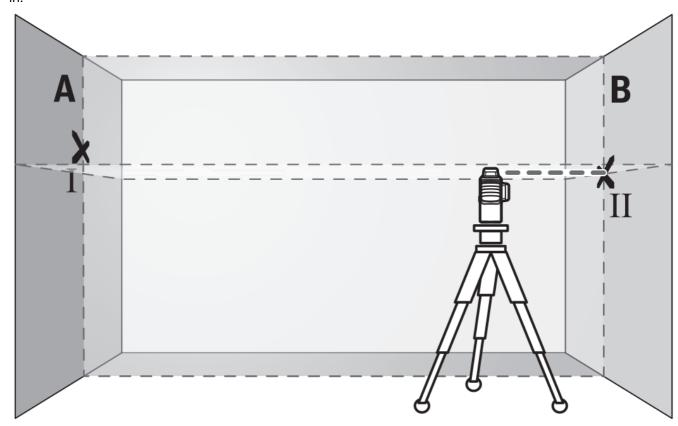
• Align the height of the measuring tool (using a tripod or by underlaying, if required) in such a manner that the cross point of the laser lines is projected against the previously marked point II on the wall B.
