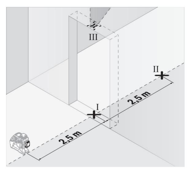
• Mark the centre of the vertical laser line at the floor of the door opening (point I), at a distance of 5 m beyond the other side of the door opening (point II) and at the upper edge of the door opening (point III).
