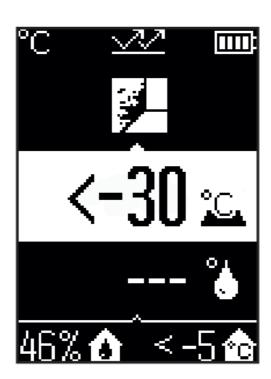
For an ambient temperature: > 50 °C (too high) or < -5 °C (too low) The values of this object cannot be measured. Aim the laser circle at another object and start a new measurement.
