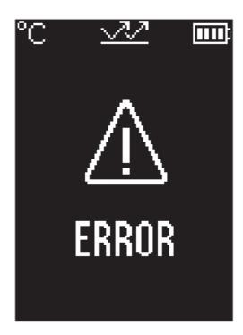
The measuring tool has experienced an internal error and switches off after five seconds. To reset the software, remove the batteries, wait a few seconds and then reinsert the batteries.
