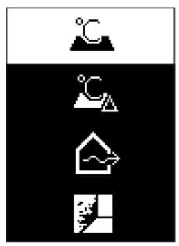
To open the mode menu, press the ON/OFF button/mode button (12). Use the ON/OFF button/mode button (12) to select the required mode. Confirm your selection by pressing the measure button (1) or the emissivity button (13).
