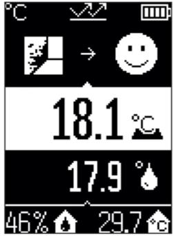
In mould warning mode, the ambient temperature and relative humidity (see "Relative humidity", page 37) are measured. The dew point temperature (see "Dew point temperature", page 37) is then calculated using these two values.
