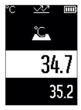
Surface temperature mode is used to measure the surface temperature of an object.
