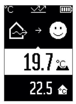
In thermal bridge mode, the surface and ambient temperatures are measured and compared with each other. If there is a significant difference between the two temperatures, a thermal bridge (see "Thermal bridge", page 37) warning is issued. Press the measure
