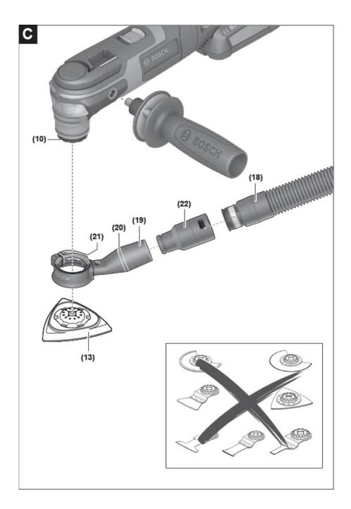
Always connect a dust extraction system for sanding. Remove the application tool and the depth stop (15) for fitting the dust extraction system (20) (accessory). Slide the dust extraction system (20) as far as it will go over the tool holder (10) onto the collar of the power tool. Turn the dust extraction system to the required position (not directly under the power tool). Push the clamping lever (21) shut to fix the dust extraction system in position.
