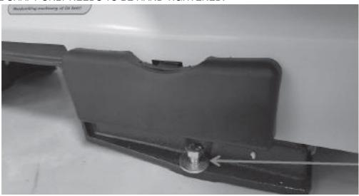
It is normal for scroll saws to create a lot of vibration. Fixing the saw down to a heavy duty work bench is recommended. Some people also find using a vibration absorbing mat helps. There are three bench mounting point provided.
