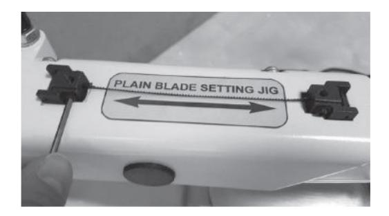
**Using plain end blades** To set the blade clamps onto plain end blades, use the setting jig located on the top arm. Loosen the grub screws on either side of the clamps then slot a new blade into each end. Tighten up the grub screws to hold the blade in place making sure it is held centrally.
