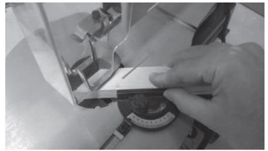
• The mitre guide can be set up to a 45 degree angle for performing mitre cuts.
