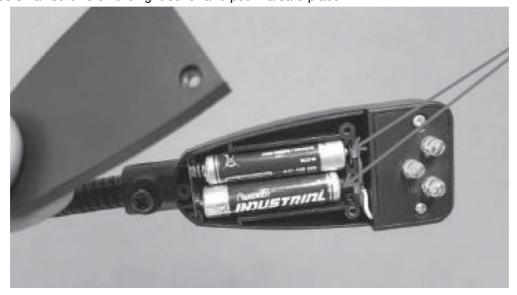
Fit the two batteries provided ensuring they are the correct way around. Replace the cover and refit the screws.
