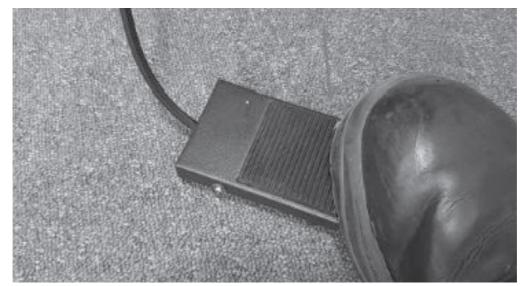
• To start the saw, press down on the foot switch. The blade will move at the set speed. Using the foot switch allows both hands to be used to guide the work piece and the convenience of stopping and starting without taking your hands off.
