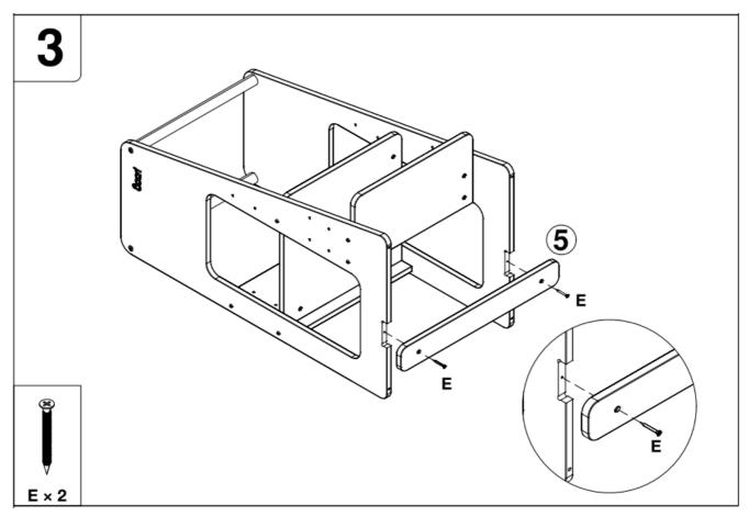
• Before tightening bolts, position the learning tower upright to ensure that it sits level on the ground.
