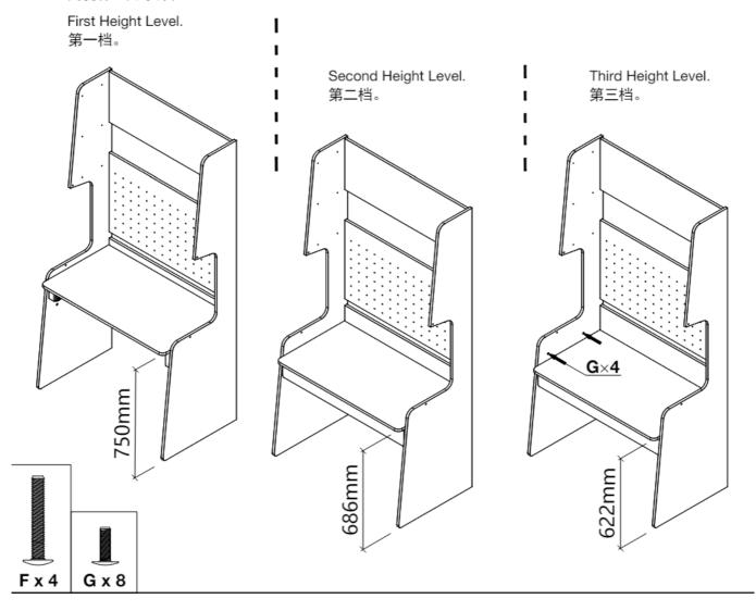
Down (下) Front (前) H x 4 Repeat process for both ends. 请用相同方法安装另外一个。 Down (下)
