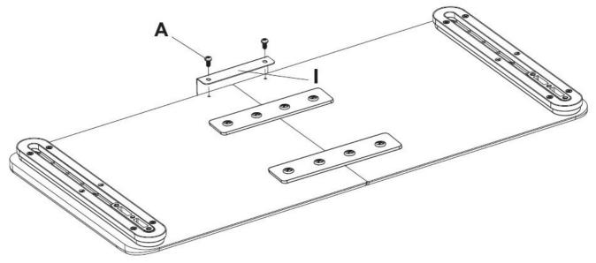
Use the ST4.2X9.S pan-head tapping screw (A) on the back of the keyboard baffle (I) to tighten the keyboard board with a screwdriver.
