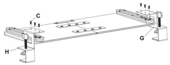
Use MSX12 round head screws (C) to install the clamps (G, H) on the slider, and tighten with a screwdriver.
