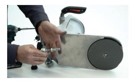
• Reinstall the new wheel and the bottom handwheel.
