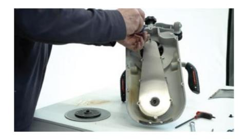
• Remove the blocking tool on the back side.
