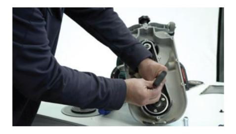
Remove the pulley by inserting the blocking tool into the hole on the machine arm and gently knock it with a hammer.
