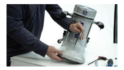
$\circ\,$  Hold the blocking tool steady while turning the sanding disc counter clockwise.
