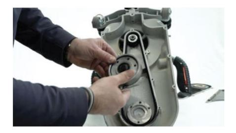
• Make sure that you place the pulley in the right position by using the blocking tool to fixate it.
