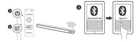
Short press "BT" button on the remote control or on the soundbar to enter Bluetooth mode. The BT will flash when entering the pairing mode, and will stop flashing once successfully paired
