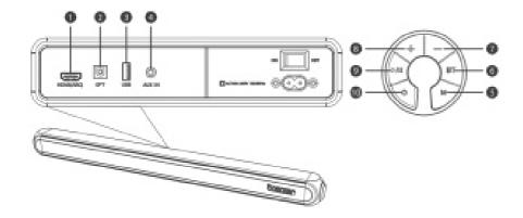
1 HDMI(ARC): Connect to compatible devices via a HDMI cable (not provided).
