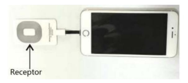
Step 2: Fixed the receptor on the back of the phone.
