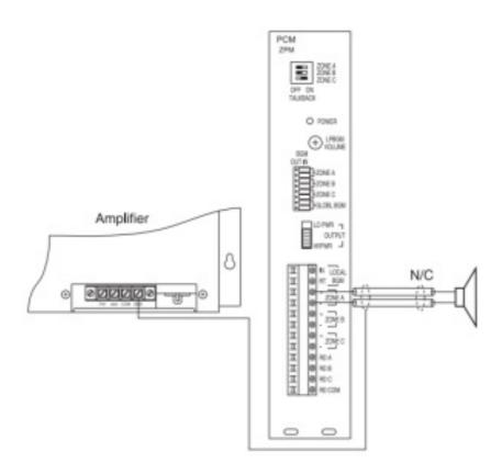
The speaker of each paging zone connects to the appropriate screw terminals on the connector block. These are labeled ZONE A, ZONE B, and ZONE C. Each connection is marked + and – as a means of identifying phasing of the zone.
