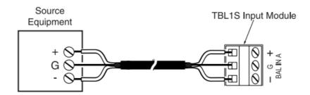
Connect the shield wire of the source signal to the "G" terminal of the input. If the "+" signal lead of the source can be identified, connect it to the plus "+" terminal of the input. If the source lead polarity cannot be identified, connect either of the hot leads to the plus "+" terminal. Connect the remaining lead to the minus "-" terminal of the input.
