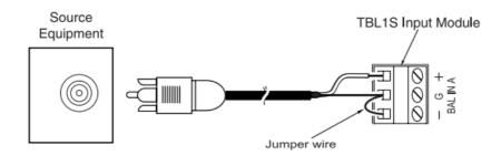
When the source device provides only an unbalanced output (signal and ground), the input module should be wired with the "-" input shorted to ground (G). The unbalanced signal's shield wire is connected to the input module's ground and the signal hot wire is connected to the "+" terminal. Since unbalanced connections do not provide the same amount of noise immunity that a balanced connection does, the connection distances should be made as short as possible.
