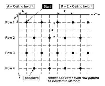
The layout of the speakers should be planned before installation begins. Layout starts in one corner of the room. The first speaker should be positioned from each wall a distance approximately equal to the ceiling height of the room.
