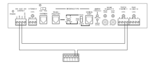
The bypass terminals override the volume control setting whenever 9V to 30V DC (at 22 mA) is applied to the D+ and D- terminals. See front page for amplifier and speaker connections.
