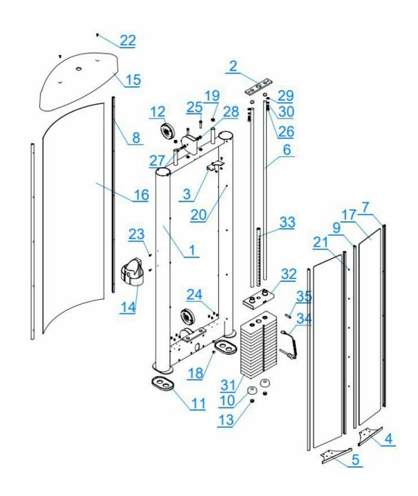
**Weight Tower Frame Assembly Guide**
